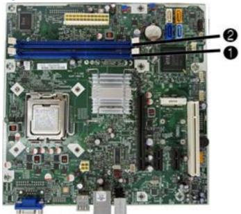
Figure 2-6 DIMM Socket Locations — 500B/510B
